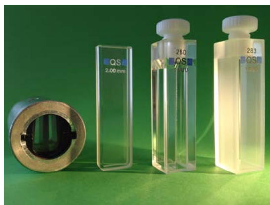
Cells made of quartz glass are used to hold biological samples for absorbance, circular dichroism and fluorescence measurements.
