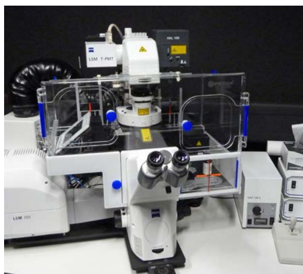
Fig. 2: Zeiss LSM700 inverted scanning confocal with incubation chamber for live imaging, large samples, and FRAP.
