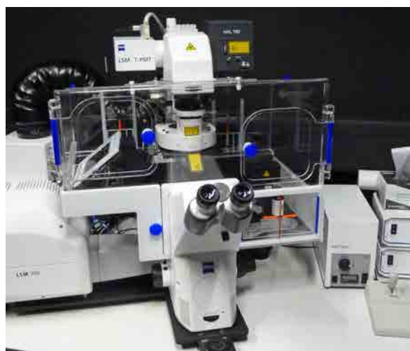
Fig. 2: Zeiss LSM700 inverted scanning confocal with incubation chamber for live imaging, large samples, and FRAP.
