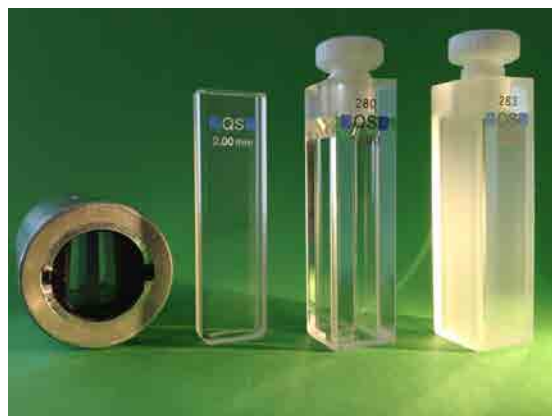
Cells made of quartz glass are used to hold biological samples for absorbance, circular dichroism and fluorescence measurements.
