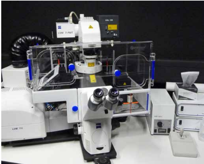
Fig. 2: Zeiss LSM700 inverted scanning confocal with incubation chamber for live imaging, large samples, and FRAP.
