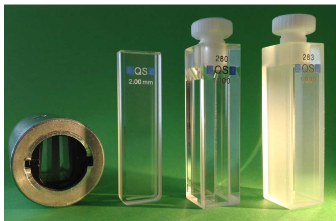
Cells made of quartz glass are used to hold biological samples for absorbance, circular dichroism and fluorescence measurements.
